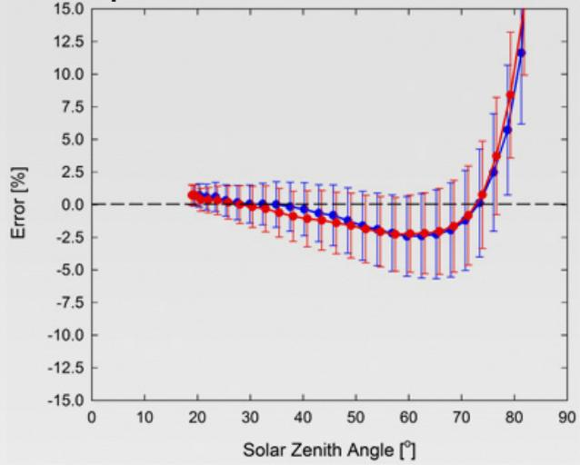
Mean cosine response of twenty-three replicate sensors (**error bars represent two standard deviations above and below mean**). Cosine response measurements were made by direct side-by-side comparison to the mean of four reference thermopile pyranometers, with solar zenith angle-dependent factors applied to convert total shortwave radiation to PPFD. Blue points represent the AM response and red points represent the PM response.
