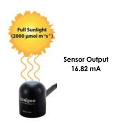
Example of PPFD measurement with an Apogee quantum sensor. Full sunlight yields a PPFD on a horizontal plane at the Earth's surface of approximately 2000  $\mu$ mol m-2 s-1. This yields an output signal of 16.82 mA. The signal is converted to PPFD by subtracting the 4.0 mA offset and then multiplying by the calibration factor of 156  $\mu$ mol m-2 s-1 per mA.
